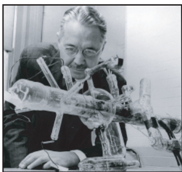
Harrison E. Farnsworth in a 1959 photo with a low-energy electron diffraction tube
