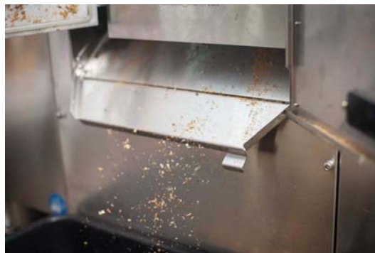
The Trisys converts waste into a dried, sterile biomass soil amendment that can be used as compost. The byproduct is easily collected in a bin.
